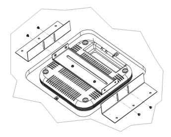
5. Fit assembly into the suspended ceiling. Attach LAN cable to the rear of the BSAP-18XX before tile is fully seated.
