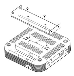
3. Slide the trim plates into the side groove just above the Kensington lock of the BSAP-18XX as shown below. Slide both plates fully in until they meet. Fasten the trim plates together using 2 M3x6mm screws.
