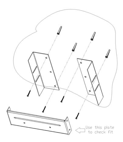
2. Fasten the rear mounting bracket to the bottom of the BSAP-18XX using 2 M2.5x7mm screws as shown below.
