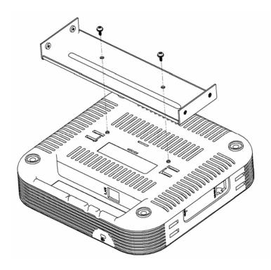
3. Attached the BSAP-18XX (with rear bracket installed) to the side brackets (mounted to the ceiling/wall in Step 1) using 4 M3x6mm screws as shown below.
