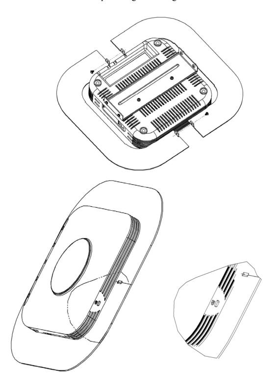
4. Lay the BSAP-18XX face down and place the cut ceiling tile over the unit as shown below. Loosely attach the side mounting brackets using 4 M3x6mm screws. Gently push down on each side mounting bracket to sandwich the ceiling tile between the bracket and trim plate. Tighten the screws.
