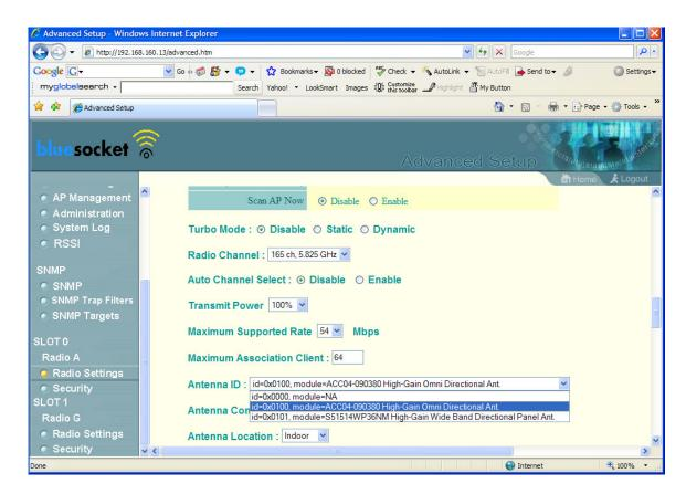
The last step on the root bridge is setting the SSID on the A radio. An SSID must be assigned to complete a link between the radios, so encryption and making the SSID blind (can be configured using the More link in Security/VAPx) should be configured as it is possible to associate to the bridge SSID. Now go the Slot 0/Radio A/Security tab to set the SSID and enable. Note: VAP 0 must be used for all bridge links. VAP 1-3 may be used for access SSIDs.
