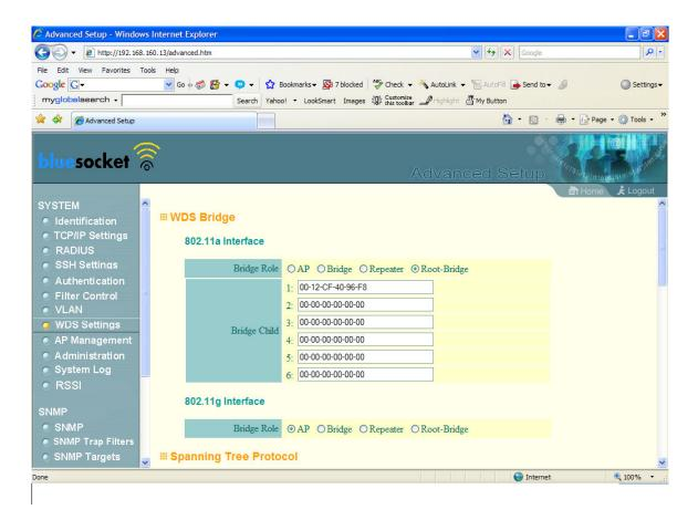
This radio is set to the root bridge and must have each child's (remote) wireless MAC in the Bridge Child fields.
