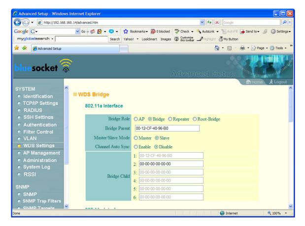
At this point reboot all radios and the bridge should come up. The BG radio may be configured on the child to test wireless access, or a hard wired device may be connected to the power injector to test connectivity.
