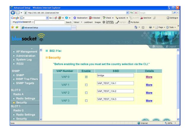
Now we configure the child (remote) radio. All the settings above will be the same with the exception of the WDS Settings. The child must be configured as a bridge and must have the **wireless** MAC of the root bridge as the Bridge parent. Must be set to slave and disable the Channel auto sync as we made it a static assignment above.
