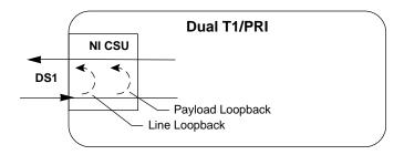
Figure 3-4. Network Loopback Test
