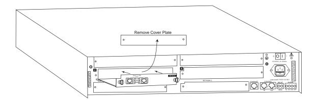
Figure 2-1. Installing the Dual T1/PRI Module
