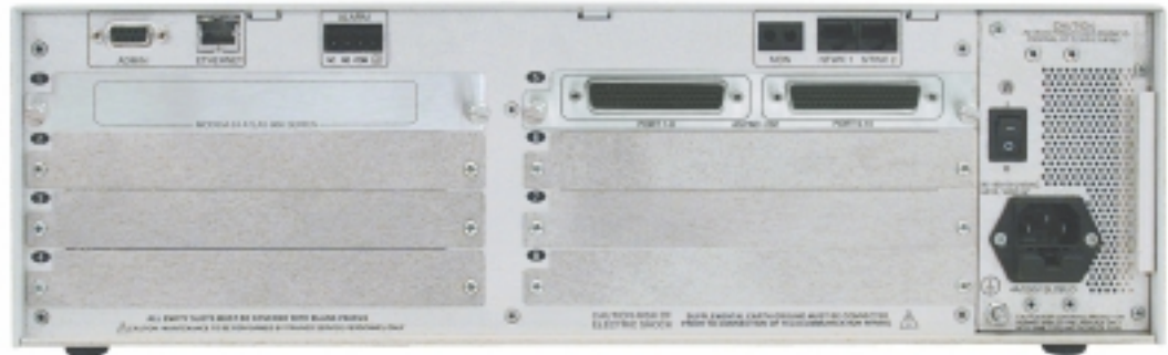
The image above shows an ATLAS 850 configured with both the Modem-24 module and the Async-232 module.
