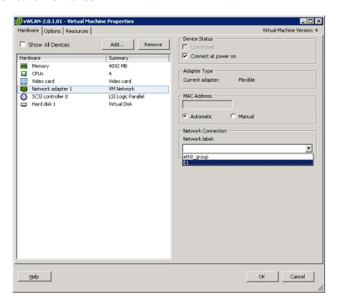
The Virtual appliances are pre-configured to support the size of your deployment. For example, if you have more than 50 access points, you will need a virtual machine with 4 cores and 4 Gbytes of memory.
