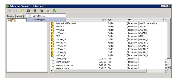
When the upload is completed, you will see the .vmx and .vmdk files – note the .vmdk file doesn't show as a –flat.vmdk file since vSphere reads the virtual disk descriptor file and represents the disk accordingly. In this example, you can remove the GettingStarted-vWLAN-VMware.pdf file since it is not needed.
