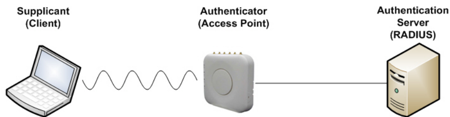
Figure 1. Components of 802.1x Authentication
