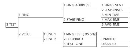
Figure 13-2. Front Panel Test Menu
