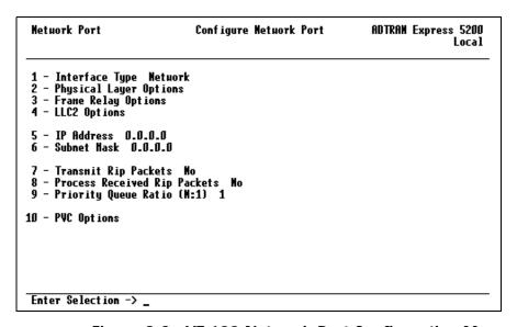
Figure 8-2. VT 100 Network Port Configuration Menu
