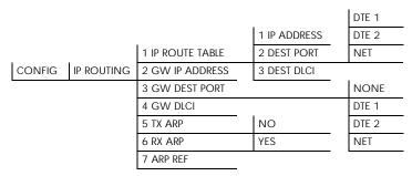
Figure 10-2. IP Routing Front Panel Menu Tree
