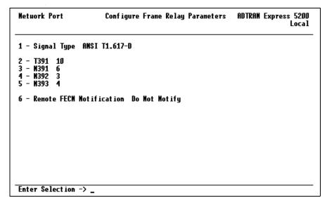
Figure 8-3. VT 100 Network Port Frame Relay Options
