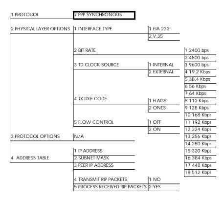
Figure 6-9. PPP Synchronous Protocol Menu Tree
