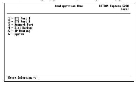
Figure 5-1. VT 100 Configuration Menu (DBU card installed)
