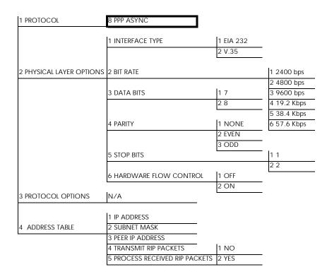
Figure 6-10. PPP Asynchronous Protocol Menu Tree
