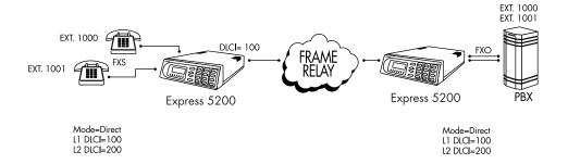
Figure 4-8. Voice Over Frame Relay Application
