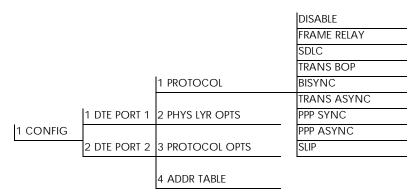
Figure 6-2. Front Panel Protocol Menu Tree
