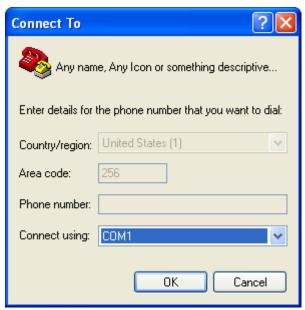
5. In the "connect to" dialog box, disregard the Area code and phone number settings. In the "connect using" pull down box, select COM1 or the COM port that your Express is attached to. If you are unsure and there is more than one COM port listed, select COM1 first.
