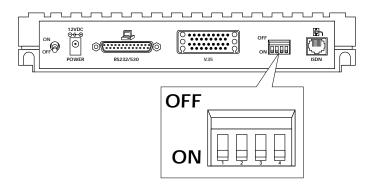
Figure 3-1. Dip Switches on Rear Panel
