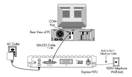
Figure 3-2. Connection Diagram
