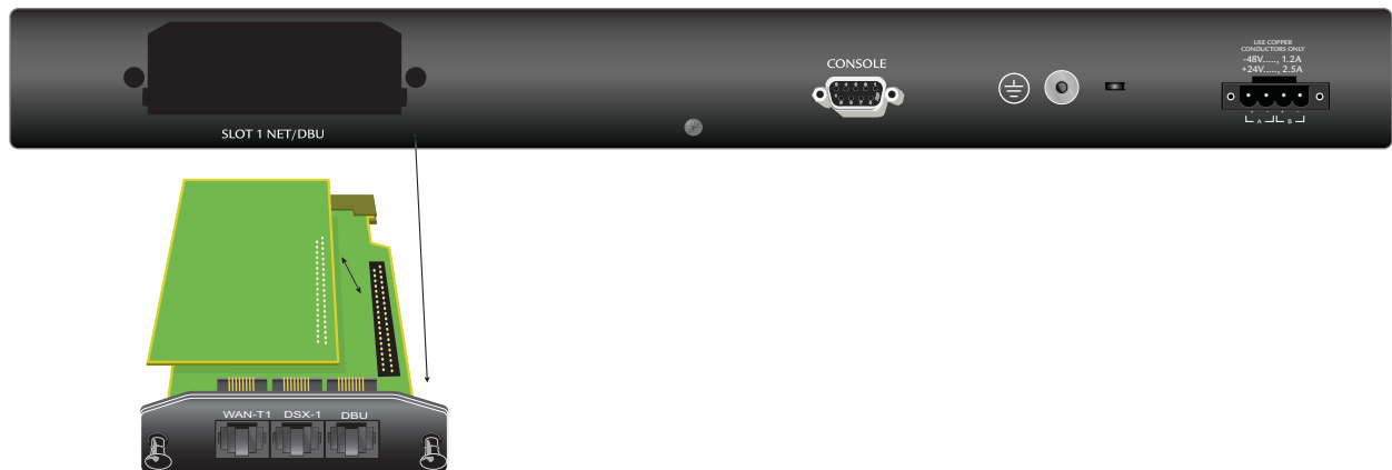
Figure 18. NIM and DIM Installation
