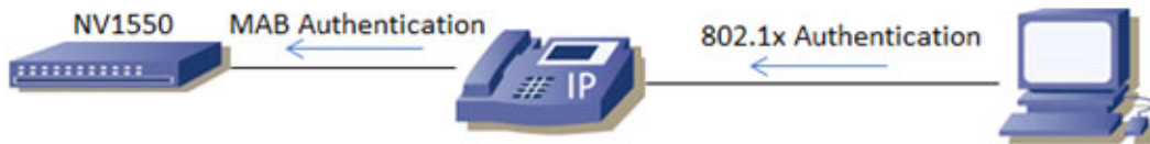
Figure 6. Voice Based Port Authentication Network Topology
