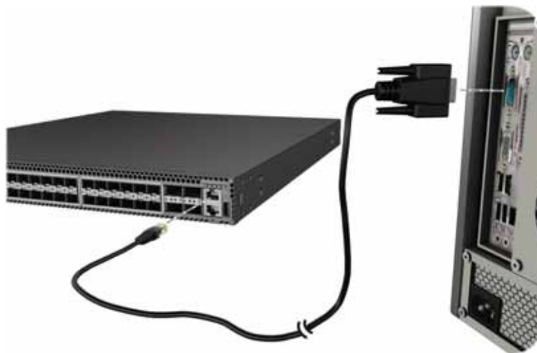
Figure 21. Console Port Connection
