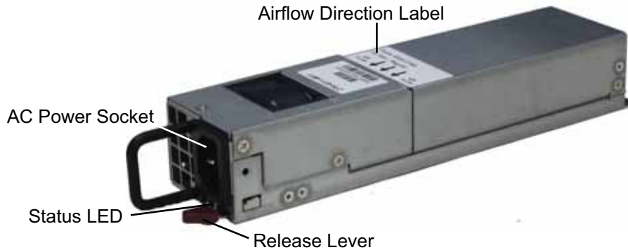
Figure 9. AC Power Supply Module
