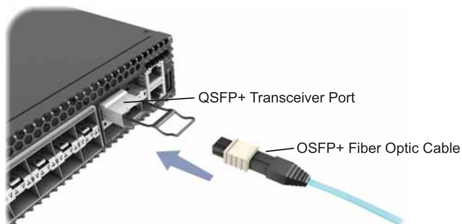
Figure 16. Connecting to a QSFP+ Transceiver
