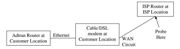
A sample configuration of a probe is shown here:
