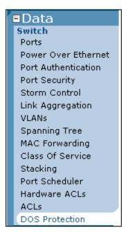
5. Select the **Configuration** tab to display the Configuration pane. This pane is the default view, and displays all DoS threat protections that can be enabled using the DoS protection feature. The threats are organized into five threat categories: **DOS L4 Header Error**, **DOS L3 Header Error**, **DOS ICMP Error**, **DOS Fragment Error**, and **Miscellaneous**.
