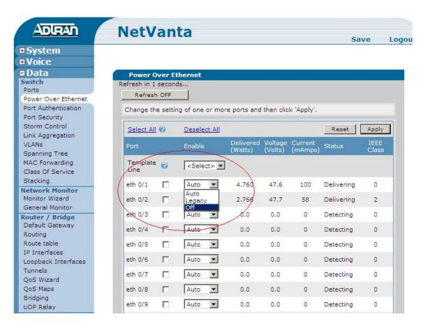
The same outcome can be accomplished using the command line interface on a per port basis by setting the port to "power inline never" and then back to "power inline auto".
