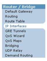
On the IP Interfaces page, select the interface that needs to be registered (make sure the IP address used is a Public Address). Click the correct IP Interface and then scroll down the next page and locate the section listed IP Settings as shown below:
