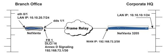
PPP over DDS Connection Diagram
