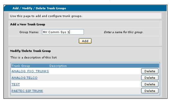
2. You will automatically be prompted to configure the new trunk group. Select **Add Members** in the trunk group's configuration, and then, using the check box, select the SIP trunk you just created. Then select **Add Selected Trunks**.
