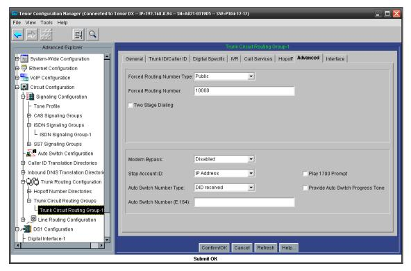
33. In **Trunk Circuit Routing Group-1**, Navigate to the **Trunk ID/Caller ID** tab. Under **Trunk ID Delivery**, choose **Calling Party Number**. Select **Confirm/OK**.
