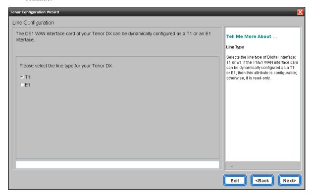
15. On the next Line Configuration screen, choose the voice coding law for the digital link. Typically, **Mu-Law** is used for **T1 links** and **A-Law** is used for **E1 links**. Select **Next>** to continue.
