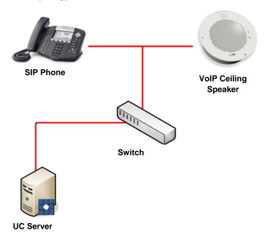
This is the network topology for a single VoIP speaker configuration. In this configuration, the ceiling speaker acts as a standalone Session Initiation Protocol (SIP) telephony device. This particular configuration does not support multiple paging zones.
