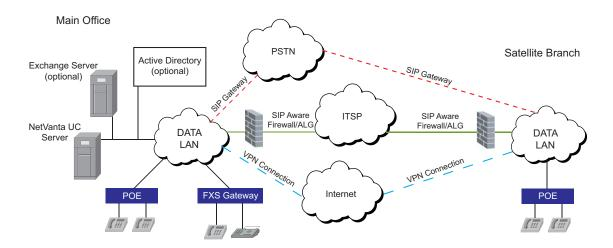
A satellite branch office implementation might involve one NetVanta UC Server at one location, and using the same NetVanta UC Server to connect to a different physical location at another branch.
