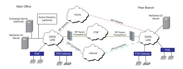
A peer-to-peer configuration might involve two NetVanta UC Servers, each configured to a different
