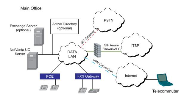
The NetVanta UC Server can accommodate telecommuters using a variety of methods. For example, telecommuters can check their voice and email messages remotely using the telephone user interface (TUI) or through Web mail, using either a VPN connection or a SIP aware firewall over the Internet.
