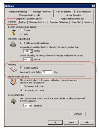
In the **Options** menu, you can enable and disable auditing logs by selecting (or clearing) the checkbox next to **Enable auditing**. In addition, you can specify for how many days records are kept. By default, audit logs keep information for **30** days; however, the valid range is **1** to **9999** days.
