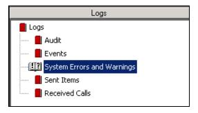
2. In the summary pane of the **System Errors and Warnings** log, right-click on the appropriate log entry and select **Accept Notifications** from the drop-down menu. Select the entry that corresponds to the error or warning notification you just received. Right-clicking on the entry acknowledges the error or warning, and the orange bar disappears from the bottom of the UC server GUI.
