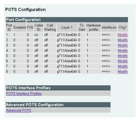
**Figure** 7a - In this example only trunk/port 1 is enabled.
