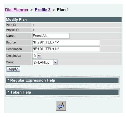
**Figure 5b** - This routes all calls from interface 9901 (SIP / UC server) to the Call Presentation Group 1001 which is a collection of trunks.
