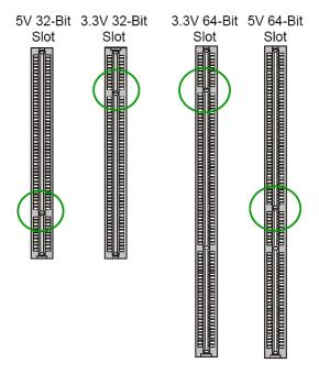
The diagrams below shows the keying for the three types of card keying for 32 and 64 bit cards (voltages refer to signaling NOT power supply):
