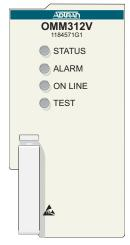
The OPTI-6100® OC-3/OC-12 Optical Multiplexer Module (OMM312V) terminates a SONET OC-3 or OC-12 fiber circuit to feed the OPTI-6100 MX or SMX chassis. It converts optical signals into digital electrical signals for distribution through the backplane to the tributary modules.
