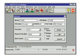
TSU devices are accessed by direct connection, in-band (ESF FDL), or modem connection.
