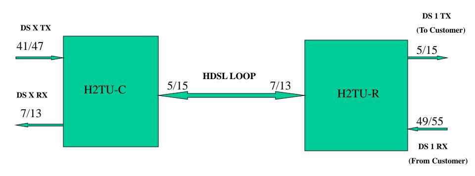
pins 5/15 connects to RJ45 pins 1/2 pins 49/55 connects to RJ45 pins 4/5
