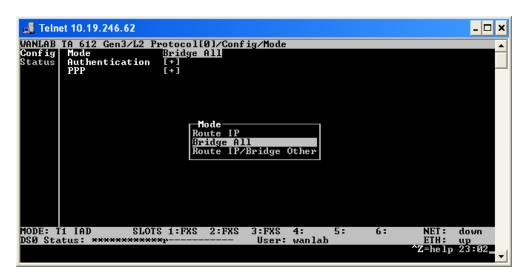
7. Arrow back to the left one time and down to Config for the Ethernet interface. Hit Enter and change the Mode there to Bridge All also. Hit H to return to the main menu.
