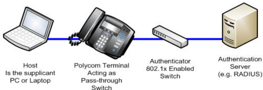
Figure 9-1: A Polycom Terminal Acting as a Pass-Through Switch
