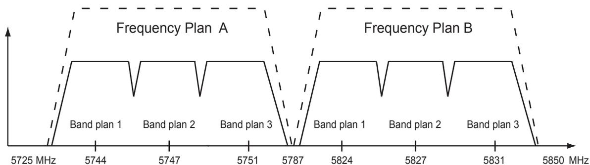
**Figure 1. 5.8 GHz Bandwidth Division (TRACER ODU)**
