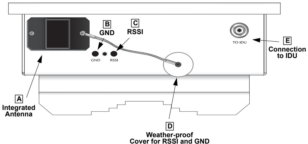
Figure 4. TRACER ODU Bottom Panel with Integrated Antenna
