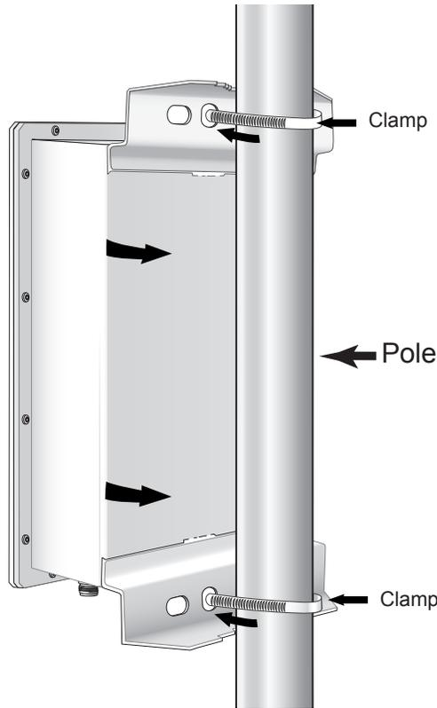
Figure 4. Mounting the Outdoor Unit (ODU)
