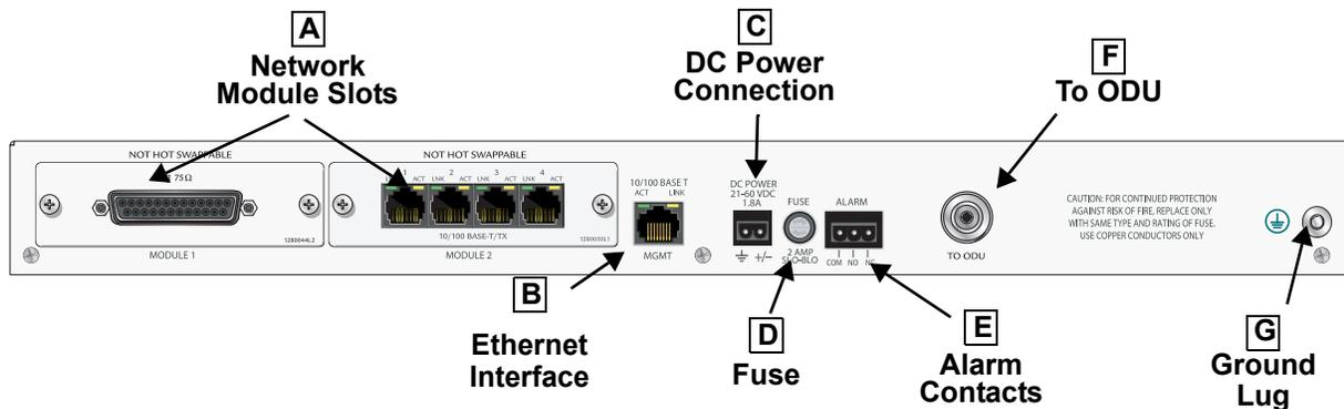
**Figure 2. TRACER IDU Rear Panel**
