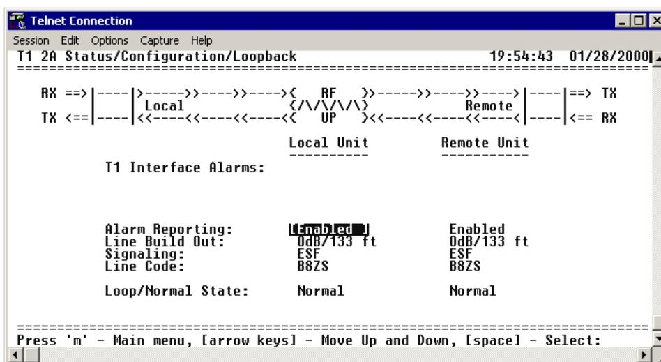
Figure 20. T1x Status/Configuration/Loopback
