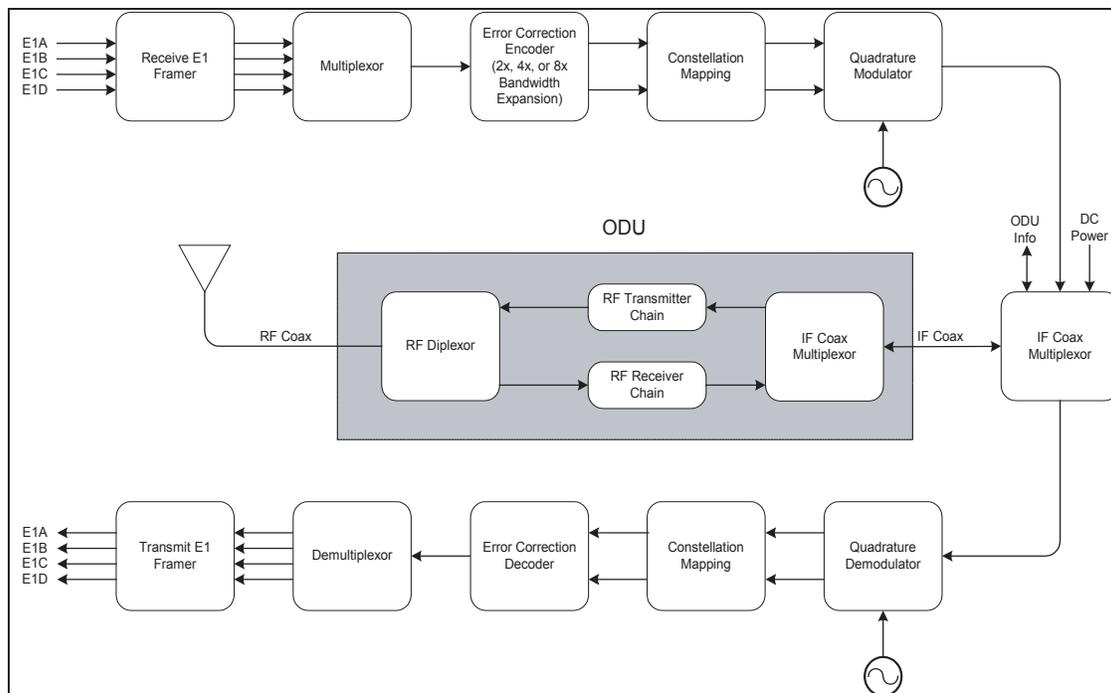
**Figure 6. TRACER 6000 Series Functional Block Diagram**
