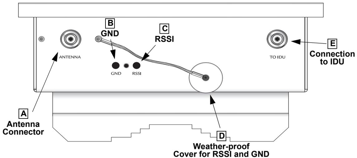
Figure 3. TRACER ODU Bottom Panel without Integrated Antenna
