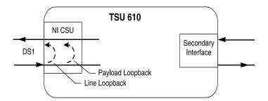
Figure 4-13. Network Loopback Tests
