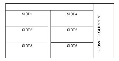
Figure 3-2. Module Slots, TSU 610
