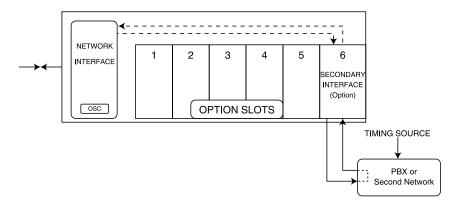
Figure 5-9. Secondary Clock Source
