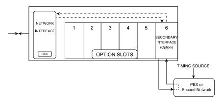
Figure 4-9. Secondary Clock Source
