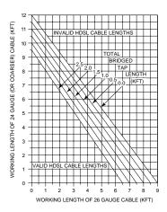
Figure F-1. HDSL Deployment Guidelines
