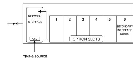
Figure 4-8. Internal Clock Source
