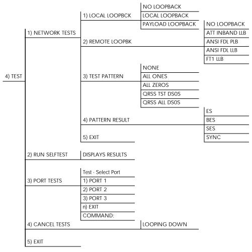
Figure 4-12. TSU 610 T1 Test Menu
