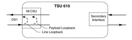
Figure 5-13. Network Loopback Tests
