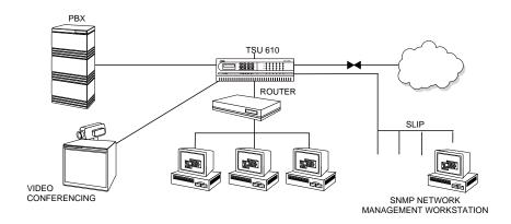
Figure 1-2. Router, PBX, Video Conferencing Application Set Up
