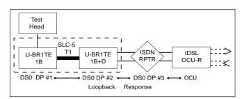
Figure 7. IDSL/DDS Loopback Response
