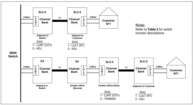
Figure 5. Position Switch Settings at Network Locations for ISDN Applications
