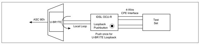
Figure 9. IDSL/DDS Remote End Initiated Loopback, Local Loop
