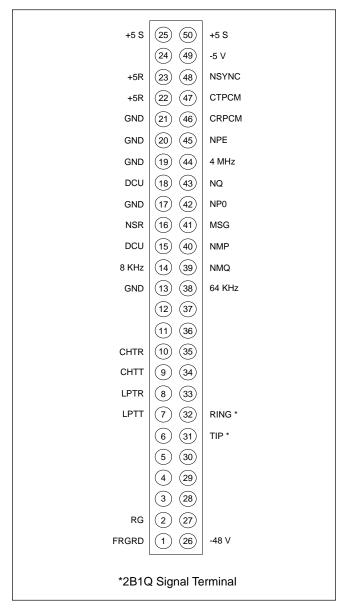
Figure 3. Backplane Pin Assignments
