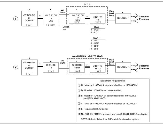
Figure 6. U-BR1TE III IDSL/DDS Circuit Diagram
