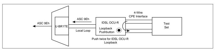
Figure 10. IDSL/DDS Remote End Initiated Loopback, Customer Loop
